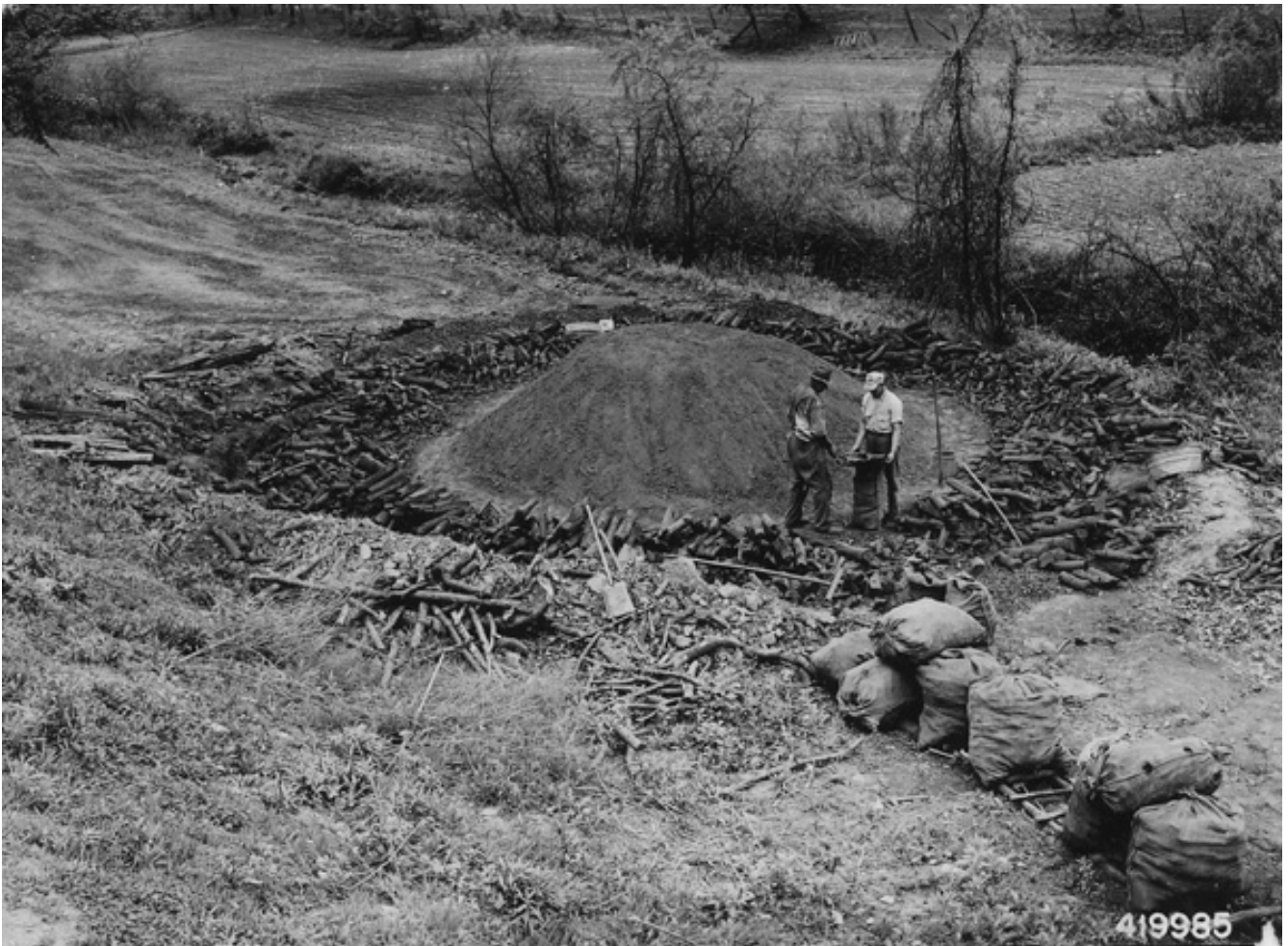
FIGURE 3. Colliers remove charcoal from the hearth. Wayne National Forest, May, 1942 (National Archives #419985).
